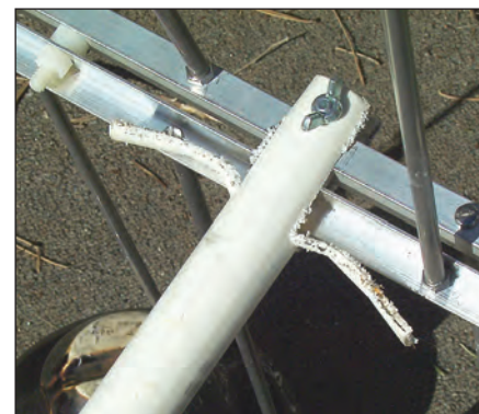
Figure 4 — Detail of PVC mast to boom attachment.
